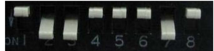
※ Please make sure to disconnect the power cable of the interface and reconnect the power cable again to apply the dip switch setting whenever changing DIP switch. Otherwise, DIP switch setting will not be applied.
