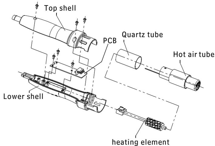
Please follow the following steps for the successful replacement of heating element of soldering station:
