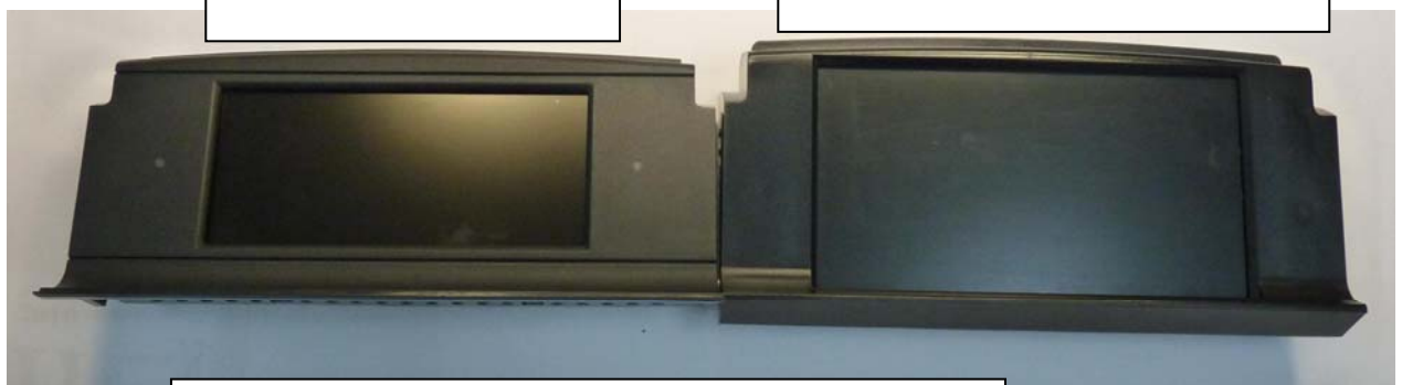
Both monitors has the same outline, same installation hooks, which makes the new one can exactly fit into the car.
