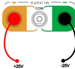
Figure 2-15 Connect +25V and -25V channel in series
