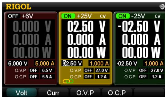
Figure 2-17 Tracking output (after tracking)
