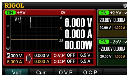
Figure 1-8 Focus waveform display mode
