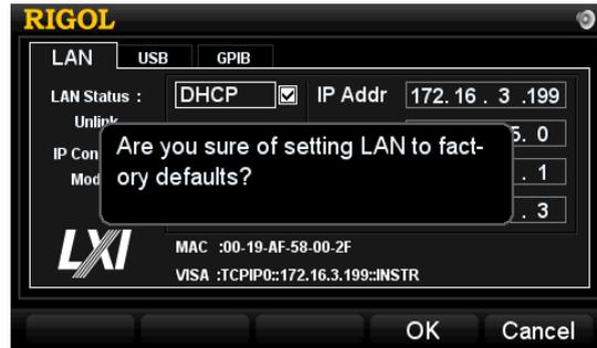
Figure 2-23 Recall the default setting of LAN
