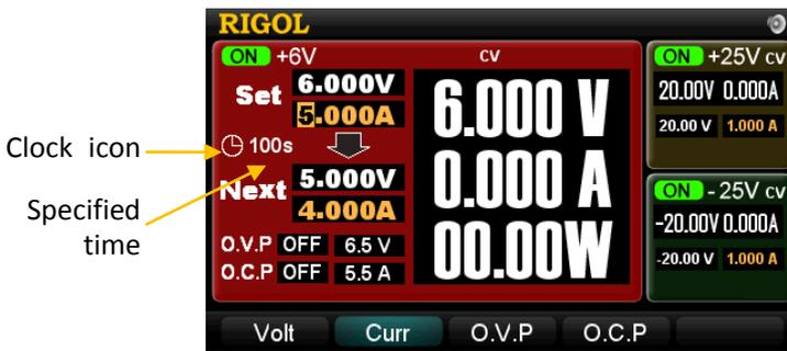
Figure 2-12 Timing output (in focus display mode)
