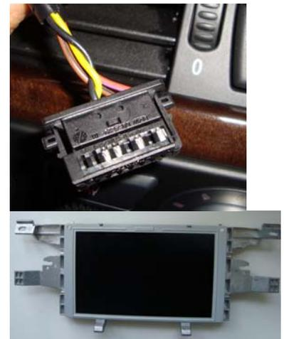
For the Audi Cars: the CD's behind can offer many control signals, when the Can box's inputs are connected there, the user may press the "mode" key on the steering wheel to switch the input. The CAN box may also be connected to the rear of air condition controller, then the driver may also get speed,reverse and light signals from the can box.
