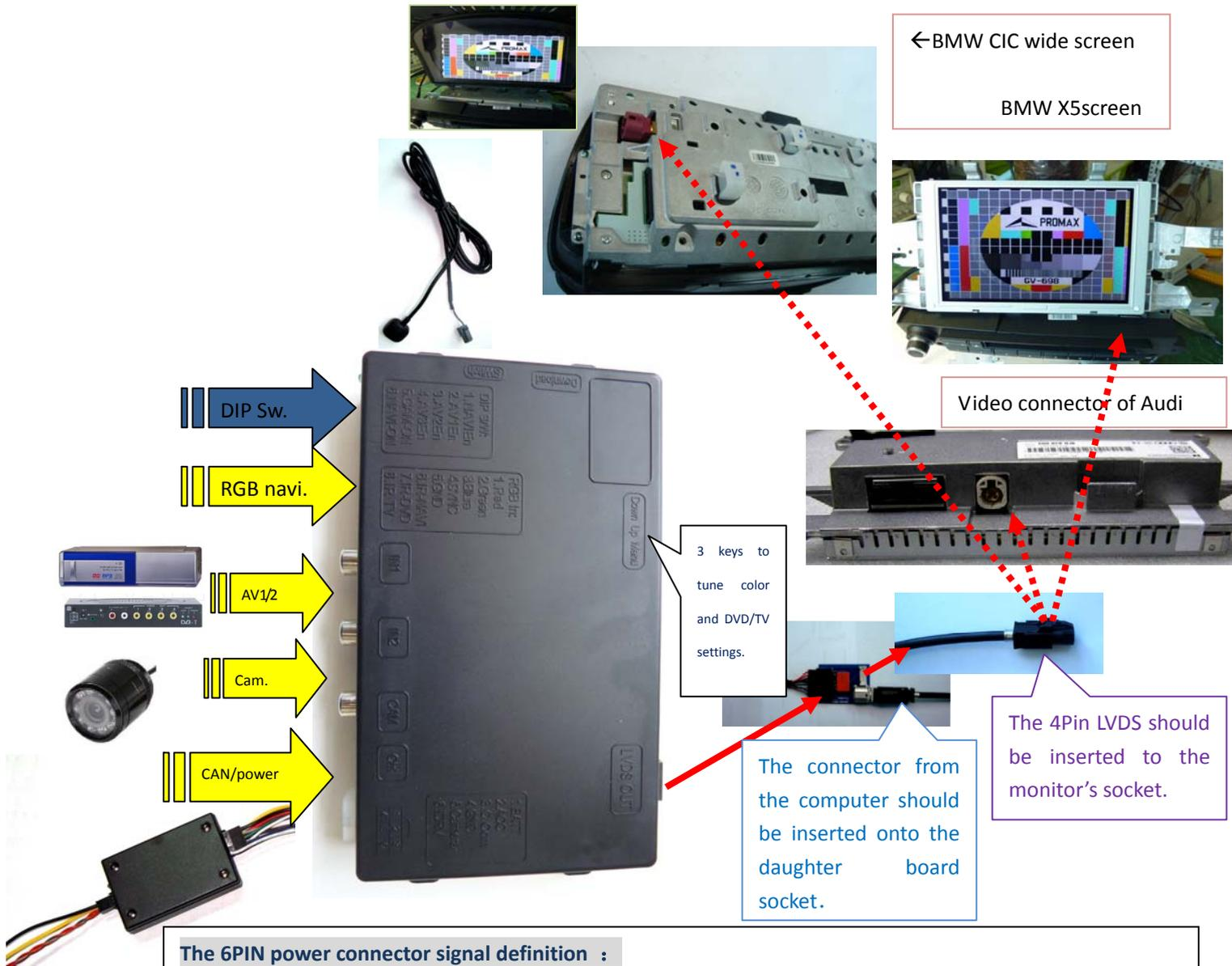
**The 6PIN power connector signal definition :**
