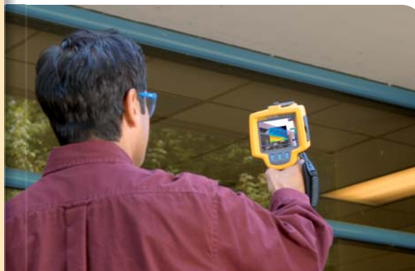
Roofing: Detect water-saturated insulation in flat-roof systems to locate damaged portions of roofing structure.
