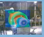
Automatic Blend A blend of the visual (visible light) and infrared image together to create a single image for optimal viewing. Easy menu options give you access to the different blending options from full thermal image to full visual image. Automatic blend provides enhanced detail to help locate problems precisely along with a visual frame of reference and helps to better focus the
