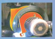
**IR/Color Alarm** Displays only temperatures falling above, below, or in between a userselected range in infrared, and anything outside the selected range as a visual (visible light) image.
