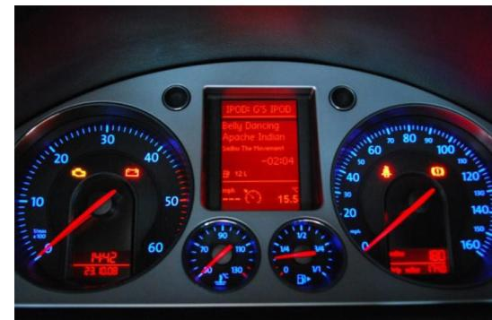
The menu of the Gateway five is displayed on the central display on the dashboard (between the two main instruments). Due to the capabilities of your car, the Gateway Five menu is not visible on the radio screen.
