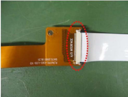
1. Connect the FFC cable to FPC cable as shown above.
