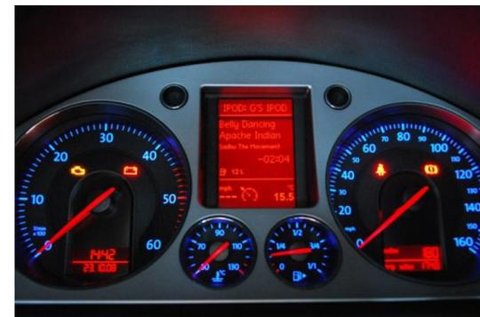
The menu of the Gateway five is displayed on the central display on the dashboard (between the two main instruments). Due to the capabilities of your car, the Gateway Five menu is not visible on the radio screen.
