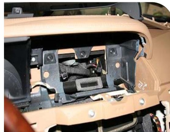
Disassemble the monitor with unscrewing the screws highlighted in red as above pictures.
