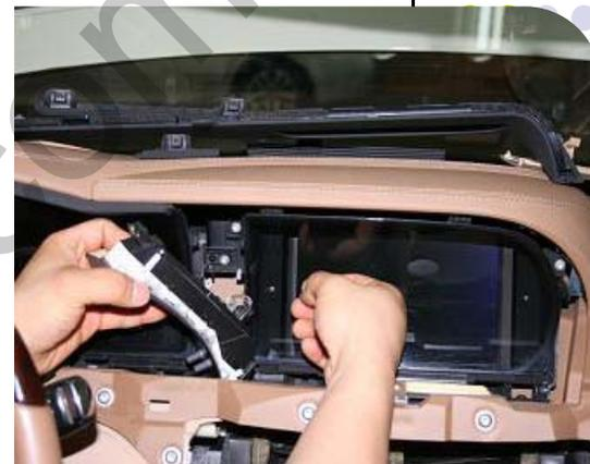
After removing the protection cover with a proper tool, unscrew the screws and pull and take apart left side of LCD.
