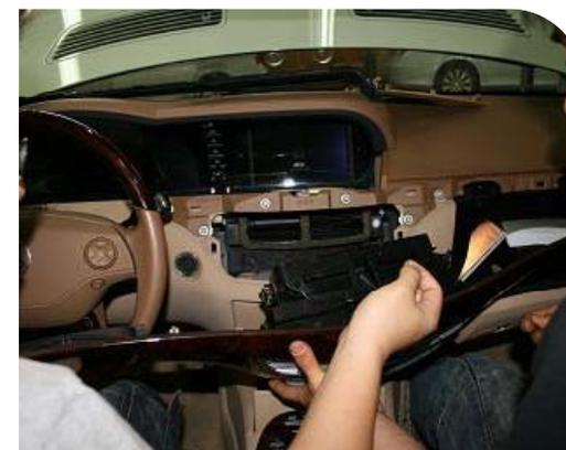
As above pictures, pull and take apart the glove box with hands after removing screws.
