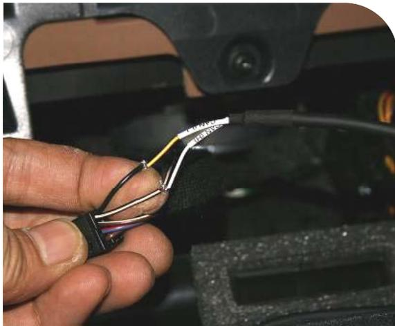
Connect supplied CAN wires to CAN wires from Car
