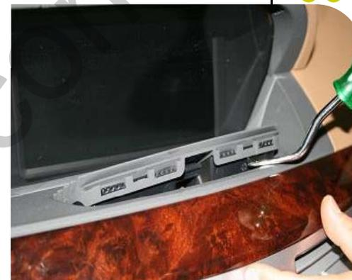
As above pictures, with a proper tools disassemble the air-con cover after removing screws on the driver's seat and passenger's seat sides.
