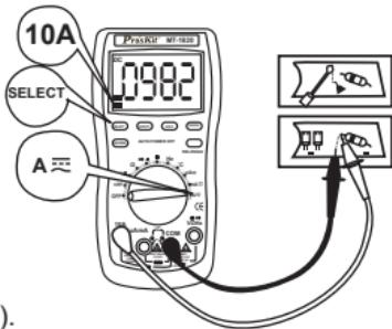
Max input current: 10A (less than 15 seconds).
