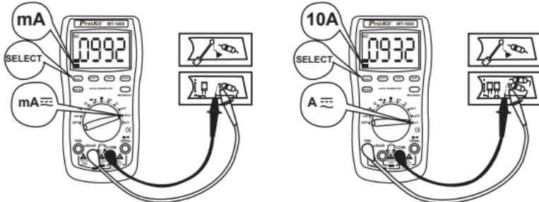
Max input current: 10A (less than 15 seconds). Overload protection: 0.5A/250V fuse, 10A/250V fuse.
