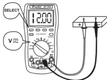
Input impedance: >60MΩ at Range 600mV , 10MΩ at other range.
