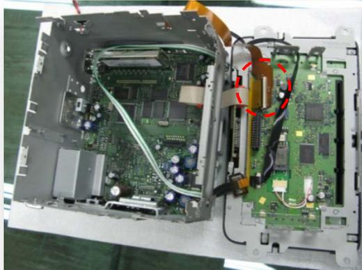
After separating LCD and Head unit board, take apart the original FPC cable.
