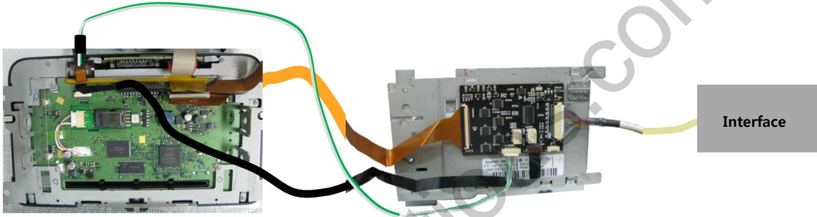
Connect Sub board with the other cables as shown above.
