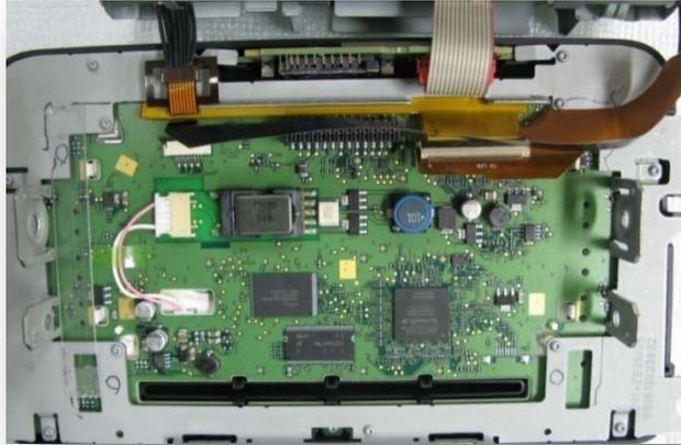
After taking apart the original touch cable from LCD side, connect the offered Touch cable. (Refer to the below how to connect)
