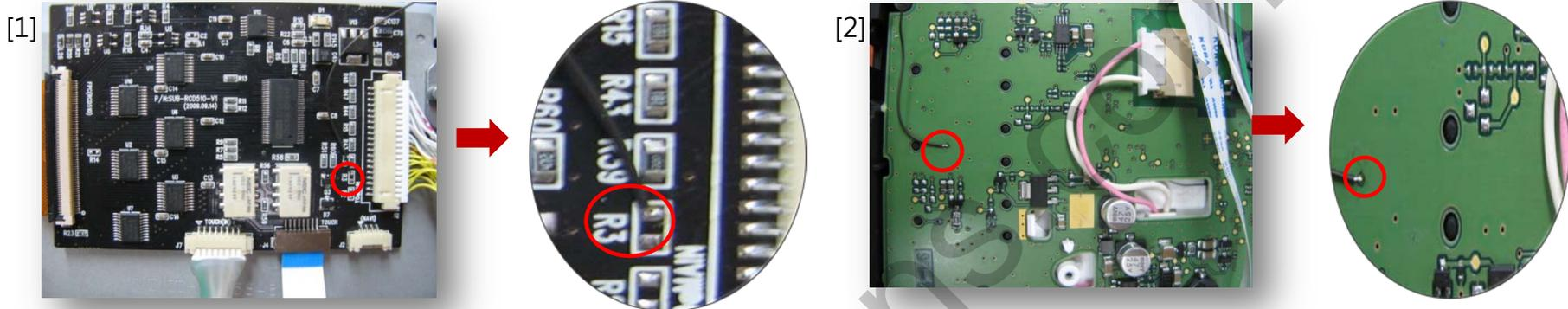
Solder a wire on "R3" in sub-board as shown left.([1]) Then solder the opposite side of the wire on an original monitor as shown right. ([2])
