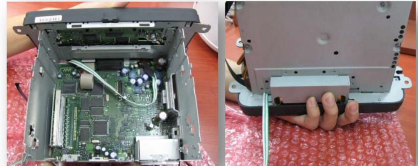
Connect Touch cable taken out to head unit side to out side as shown above.
