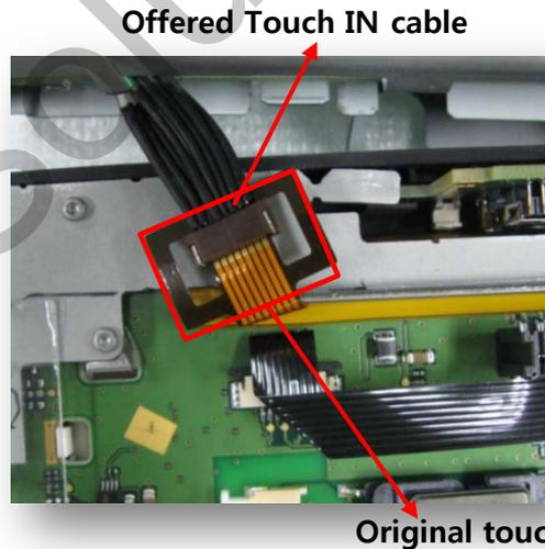
Insert the offered "Touch Out" Cable to the original connector as shown left.
