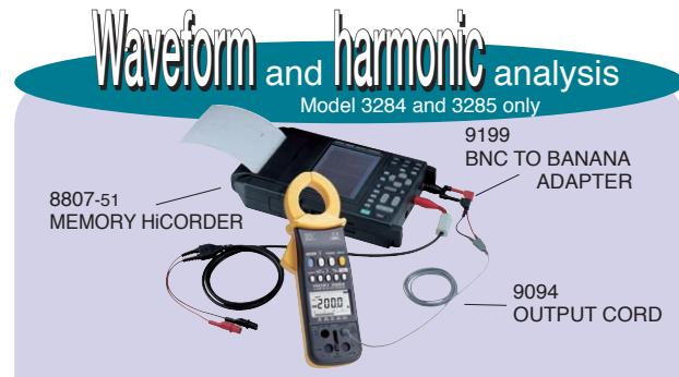
Using the external output functions of the 3284 or 3285 in combination with a HIOKI MEMORY HiCORDER enables recording of current and frequency fluctuations and recording and harmonic analysis of instantaneous waveforms. The monitor output (MON) spans a wide frequency range from DC to 20 kHz (15 kHz in the case of 3285), which allows the units to be used for electric current analysis in various fields ranging from batteries to inverters.
