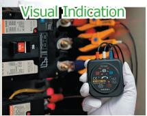
Based on the electrostatic induction theory, the 3129 series Phase Detectors can safely and accurately detect phase sequence in three-phase circuits. Correct sequence is indicated by a crystal clear beeping tune, while bright red LEDs show sequence direction.
