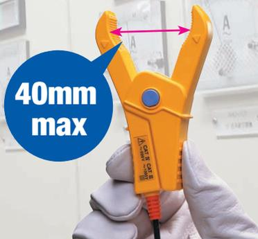
**Clamp thick conductors from 10mm to 40mm**
