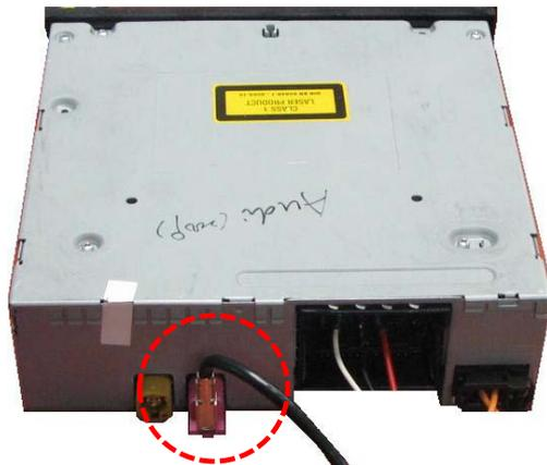
Connect Factory LCD cable from DVD Unit to sub-board ("LCD IN")
