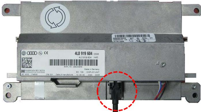
Take apart LCD monitor and factory LCD cable from LCD monitor.
