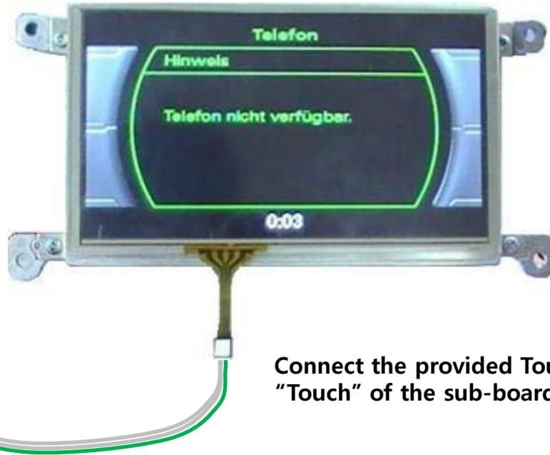
Connect the provided Touch Screen Cable to "Touch" of the sub-board and Touch Screen.
