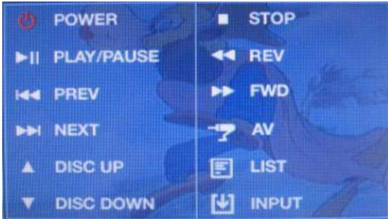
On AV1 mode, once touch the screen, Menu window appears like left picture. If no action for 5 sec or touch any other parts of the screen, this will disappear.
