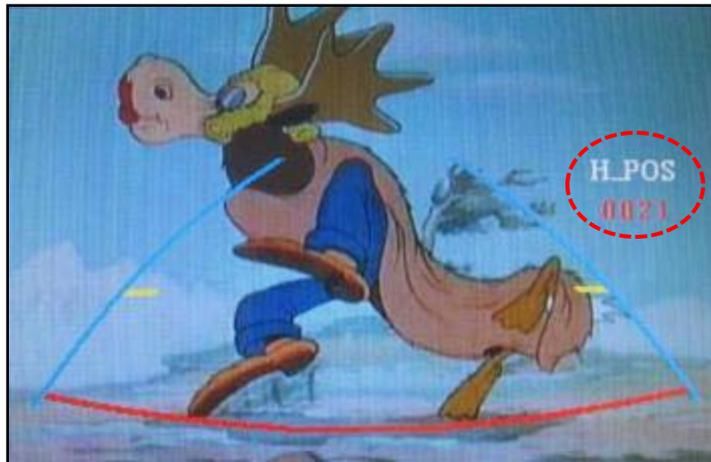
② After the setting done, rear parking guide line will appear in rear gear position. Once press "OK" button, "H\_POS" appears at the right and can adjust the line's position.
