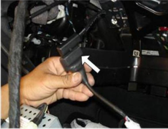
9. Connect the provided LCD cable to OEM cable from Command.
