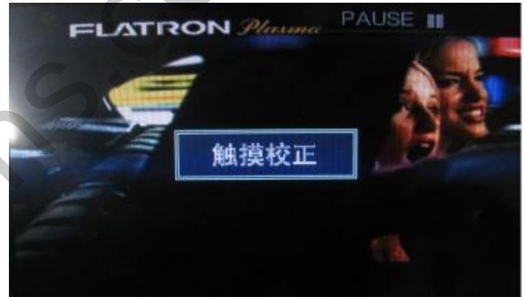
① First of all, press ◀ button on remote control 2 seconds long. Then you can access to the FACTORY mode.
