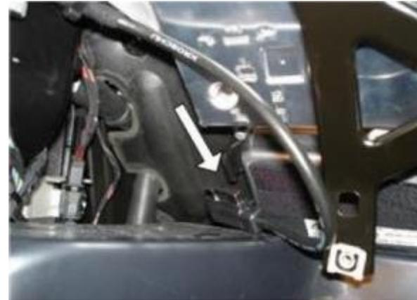
8. Separate the cable from the car
