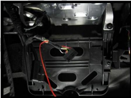
③ Connect Navi orange wire from Power cable to the 16<sup>th</sup> pin of the connector.
