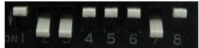
※ Please make sure to disconnect the power cable of the interface and reconnect the power cable again to apply the dip switch setting whenever changing DIP switch. Otherwise, DIP switch setting will not be applied.
