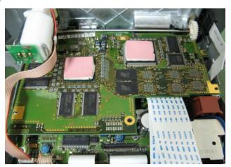
2. The connector which is pulled out the original FFC cable connect with second offered FFC cable. (The other side of second offered FFC cable connect with offered sub-board "LCD IN"
