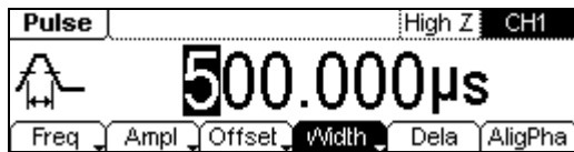
Figure 2-13 Pulse Signal Parameter Setting Interface
