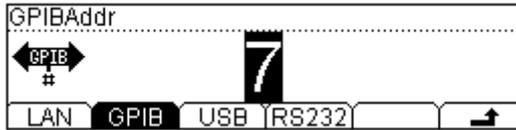
Figure 2-82 GPIB Setting
