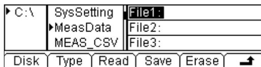
Figure 2-73 The U-Disk Storage Interface
