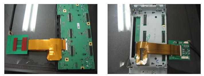
3) After the ribbon cable connection, assemble the LCD Panel and the board again. Like the photo, the interface should be connected while assembling.
