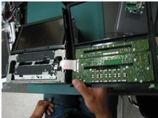
STEP 4: Carefully separate the ribbon cable.
