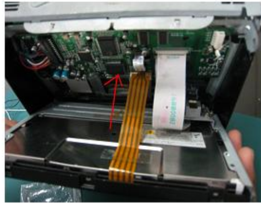
STEP 15: Connect the Original Cable to the LCD as shown in the picture
