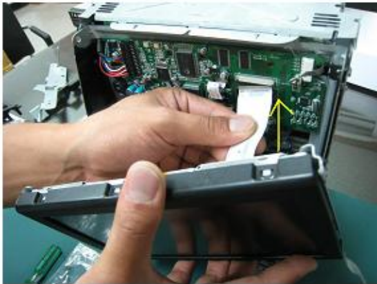
STEP 15: Connect the Original Cable to the LCD as shown in the picture
