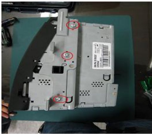
STEP 2: Screw off the star bolts front of the monitor.
