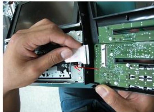
STEP 3: Take out the Plastic cover in front.
