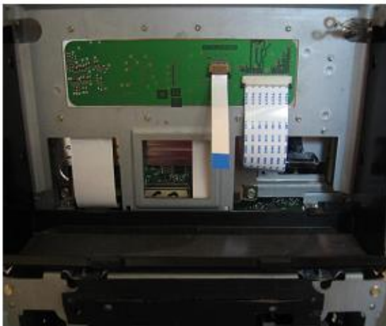
STEP 8: Slot supplied Cable in to the disassemble place.
