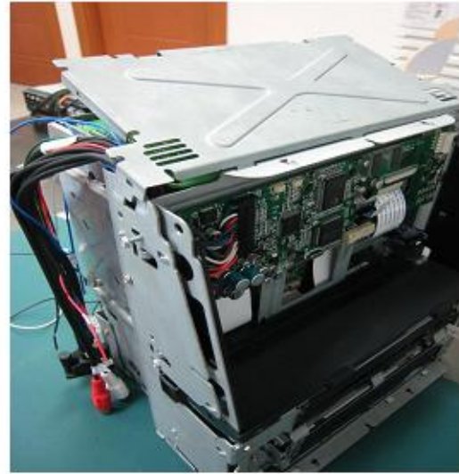
STEP 14: Reassemble the Cover.
