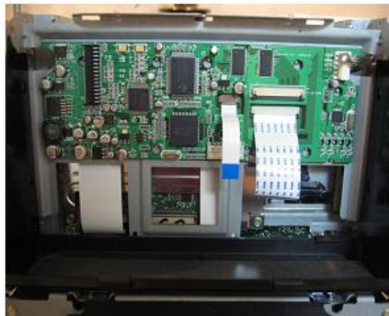
STEP9: Mount the INTERFACE.
