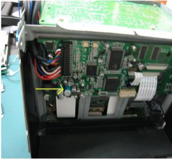
STEP 13: Route the connected cable as shown the picture.
