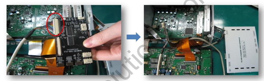
1) Connect LCD cable from Interface to sub-board.
