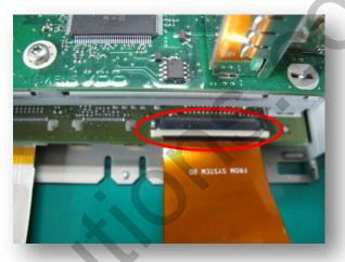
Disassemble Head Unit as shown left.
