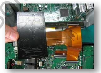
Connect the other side of FPC cable to the connector from LCD. (as shown left) Connect FPC cable to subboard. (as shown right)
