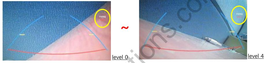
③ The width of the rear parking guide line has 5 level( $0\sim4$ ). After you control the level with "UP", "DOWN" button on the keypad, you can move to the horizontal positioning mode after pressing "SEL" button and saving process. (The current state is displayed right-top.)
