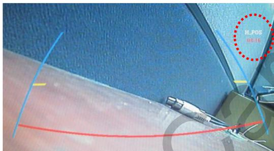
③ After Step. ② , press ▲, ▼ buttons on the Remote control to control left, right position with pressing 'OK' button, and then you can control up, down position. (Able to control 0~255)
