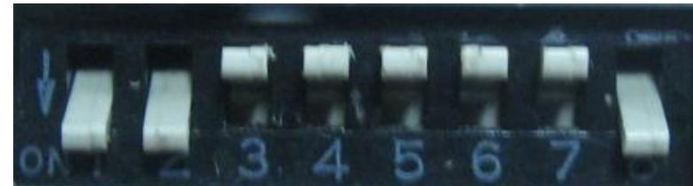
※ Please make sure to disconnect the power cable of the interface and reconnect the power cable again to apply the dip switch setting whenever changing DIP switch. Otherwise, DIP switch setting will not be applied.
