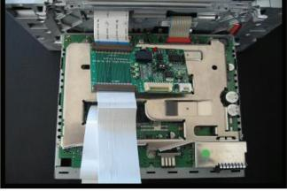
3. Take the flexible Wire and connect it to LCD OUT on the interface board.
