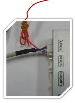
Solder the Orange wire on Mode cable to the Head Unit like picture
