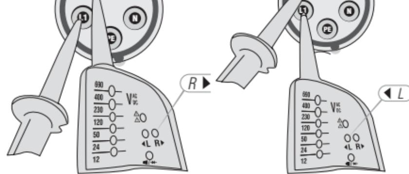
▶ R ➤ signifies that the supposed phase L1 is the actual phase L1 and the supposed phase L2 is the actual phase L2
