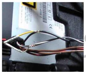
Connect the original CAN wire to the offered CAN wire as shown left.
