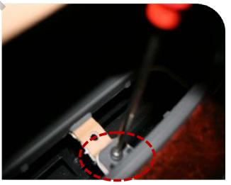
After detaching the air-con cover, remove the inside screw with a tool like the pictures.
