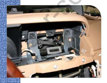
The monitor is removed from the car.
