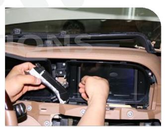
Remove the screw marked on the left picture, pull the left part out from the monitor like the right picture.
