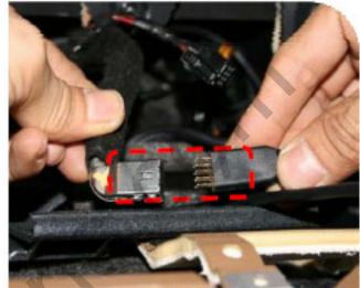
Connect LCD Out cable coming from the car with LCD-In cable offered with right position like the picture.
