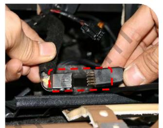
Connect LCD Out cable coming from the car with LCD-In cable offered with right position like the picture.
