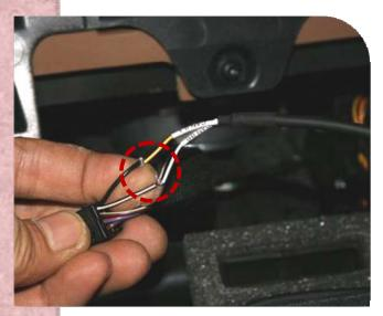
Wire offered CAN wires with CAN wires of the car. White+Black: CAN HIGH Black: CAN LOW
