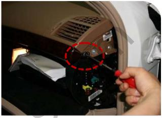
Remove the screws of driver's seat ward, passenger's seat ward on the glove box with proper tools.
