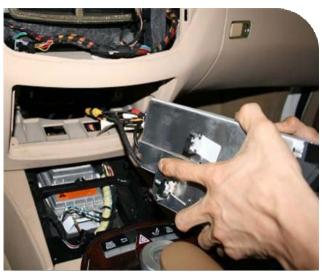
Remove the screws and take Head unit out from inside.
