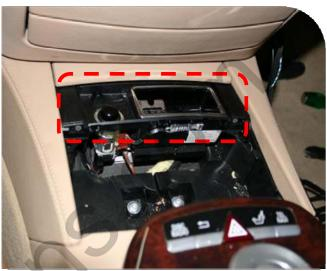
Remove the cup holder with screws.
