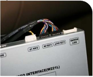
Picture with all cables connected on the interface.
