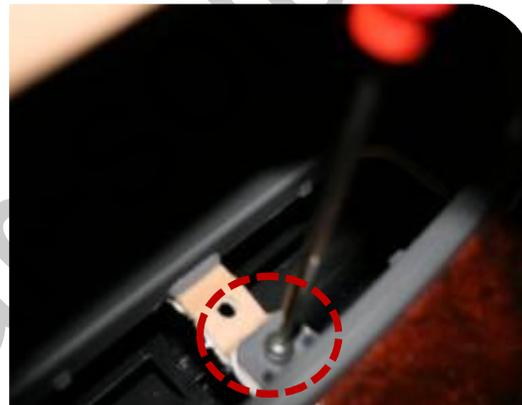
After detaching the air-con cover, remove the inside screw with a tool like the pictures.
