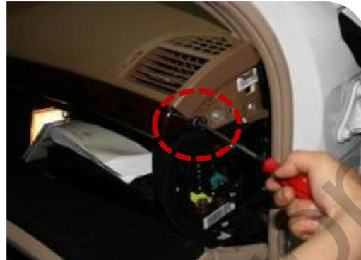
Remove the screws of driver's seat ward, passenger's seat ward on the glove box with proper tools.
