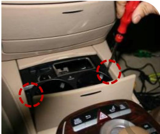
Remove the cup holder with screws.
