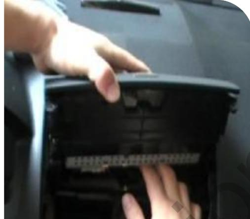
Take the monitor out from the car after removing the screws. Be careful with the cable connected to the monitor.
