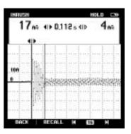
• Inrush current up to 500A with supplied current probe
