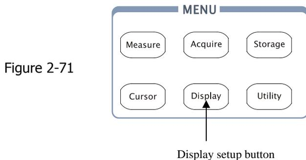
Press the Display button to pop up the menu for the settings of the display system.
