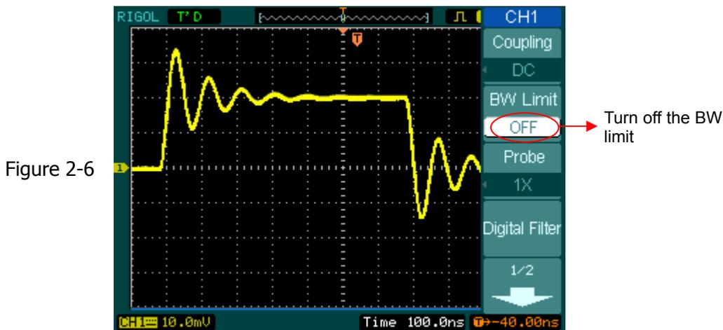
Press **CH1**→**BW Limit**→**ON**, to set up bandwidth limit to “ON” status. It will reject the frequency component higher than 20MHz.
