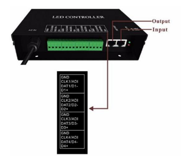
GND and DAT are for chips like TM1812, WS2811, WS2812.
