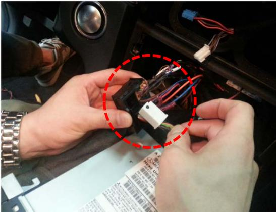
① Separate white connector cable from bunch of cable behind of Audio deck
