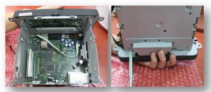
Connect Touch cable taken out to head unit side to out side as shown above.
