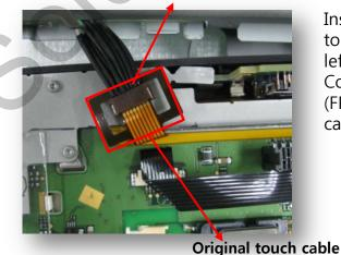
After taking apart the original touch cable from LCD side, connect the offered Touch cable. (Refer to the below how to connect)
