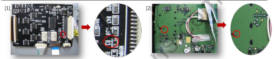
Solder a wire on "R3" in sub-board as shown left.([1]) Then solder the opposite side of the wire on an original monitor as shown right. ([2])
