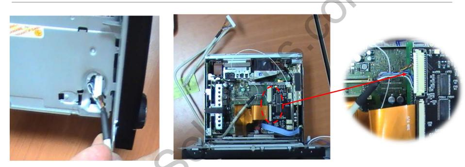
Put LCD cable into Head unit, connect sub-board and interface board.
