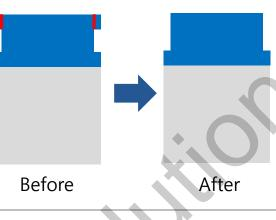
Trim edges of the original FFC cable which is connected between head unit board and monitor as shown left. (This is to connect the offered Button cable, be sure not to damage PIN on the cable. )
