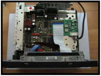
10) Connect FCC cable from LCD to SMALL BOARD LCD OUT and then connect to the RGB CONVERTER.
