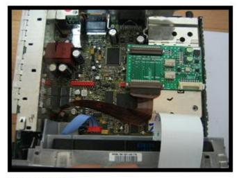
9) Connect original FCC Cable to MAIN IN on the SMALL BOARD.
