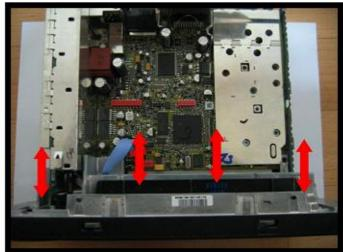
6) Unscrew the 2 bolts and detach the LCD from the body of the Commend.
