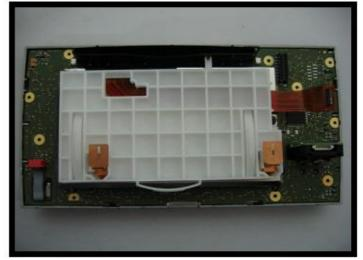
7) Unscrew 10 bolts and remove the LCD cover.
