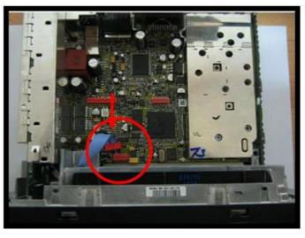
5) Detach the original FCC Cable from the board then detach the Connector. (Attention required for the delicate FCC cable.)
