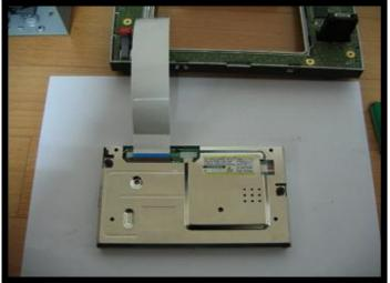
8) Disconnect the original FCC cable. Connect the supplied FCC cable to the board.
