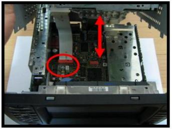
4) Lift up the front cover of the Commend. Disassemble the Connector then disassemble the cover completely.
